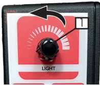
Fig. 37: Reducing the illumination level with the light controller
